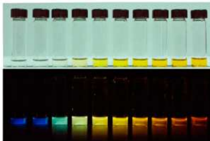
Figure 2. Visible light illuminated (top) and short-wavelength UV light illuminated (bottom) CdSe QDs from procedure 1. The reaction time increases from left to right.
